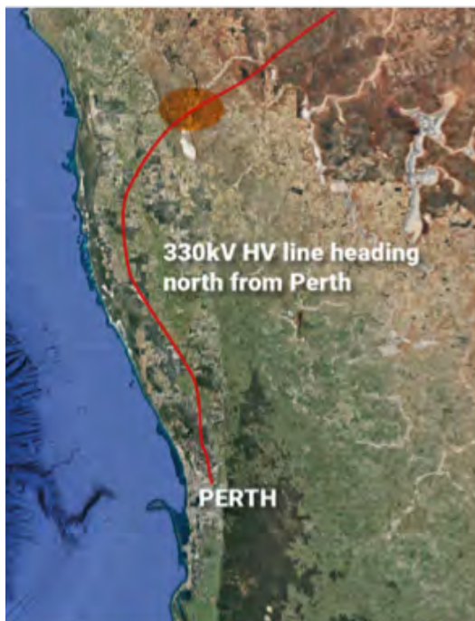
FIGURE 14 SOUTH-WEST INTERCONNECTED SYSTEM (SECTION)
